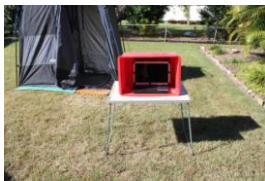
Minimum setup for a laptop. In a box with red gel cover
